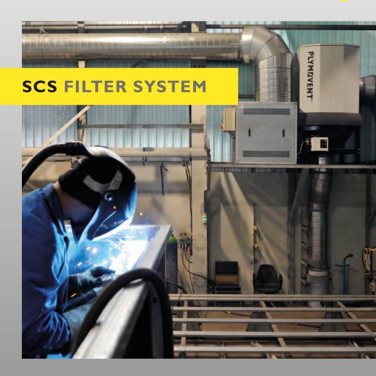
Self-cleaning filter system removes welding fumes efficiently
