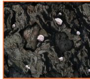
The **APCO matrix** is a grid composed of a proprietary mixture of activated carbon infused with titanium dioxide.
