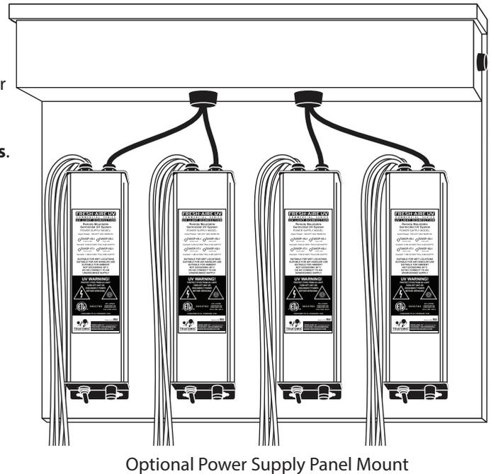
**IMPORTANT! Connect in accordance with all state and local electrical and building codes.** Proper voltage is automatically selected by the unit between 120 or 230 VAC Single Phase 50/60 hz. **IMPORTANT! External power suppressor may be needed if power surges occur.**
