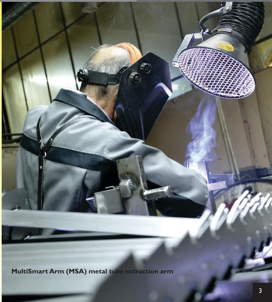
MultiSmart Arm (MSA) metal tube extraction arm
