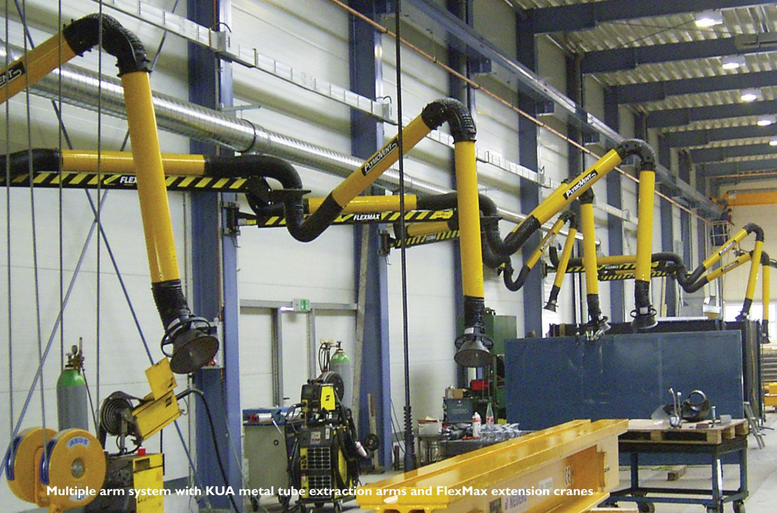
Multiple arm system with KUA metal tube extraction arms and FlexMax extension cranes
