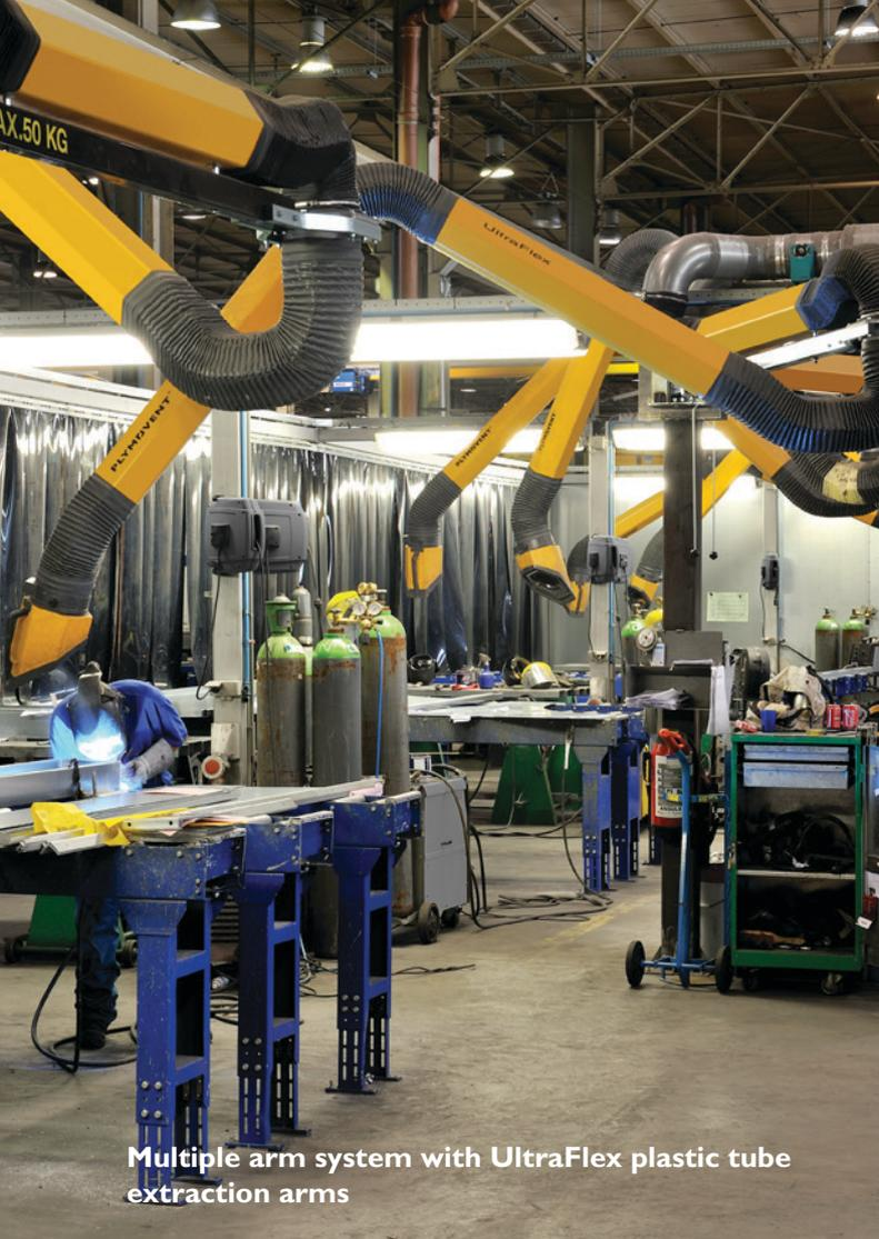
Multiple arm system with UltraFlex plastic tube extraction arms
